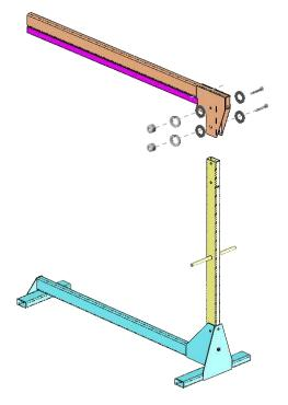
Insert the 140mm long adjustment screw (B) and flat washer (D) through the rear mounting hole in the boom. Place flat washer (D), split lock washer (E), and hex nut (F) on the screw. Tighten the adjustment screw until the boom is roughly level. Cinch the 2 side screws to temporarily hold. <a href="#">Any boom adjustment requires the 2 side-mounting screws to be loosened.</a>
