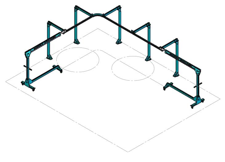
NOTE: - TOTAL WIDTH AND DEPTH SHOWN IS MINIMUM RECOMMENDED - DIMENSIONS SHOWN ARE FOR 'MEDIUM' OFFSET FLOOR STANDS - FLOOR STAND CLEARANCE: SHORT=  $\emptyset$  48", MED=  $\emptyset$  72", LONG=  $\emptyset$  96"
